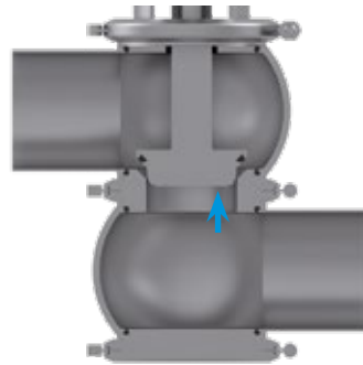
Control valve with equal-percentage control cone
