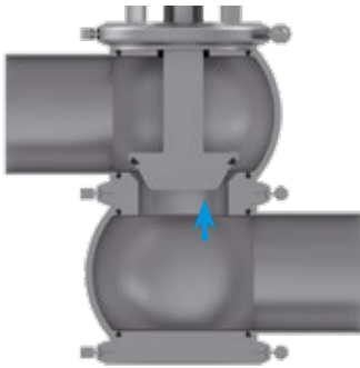
Control valve with linear control cone
