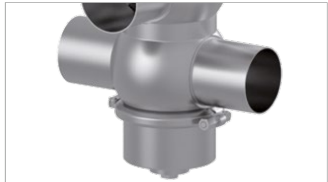
If there is cleaning media in the upper pipeline, the upper valve disc can be lifted up to allow the surface of the seal and the leakage chamber to be cleaned.
