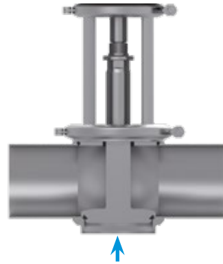
Valve type N (Spring-to-close, NC)
