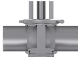
Simple shut-off with only one seal
